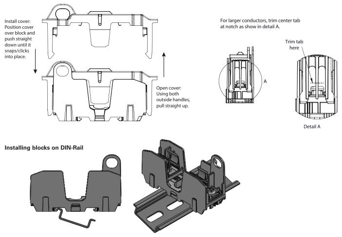
Place one edge of DIN-Rail in fuse block base, then rotate block down until it clicks into place.
