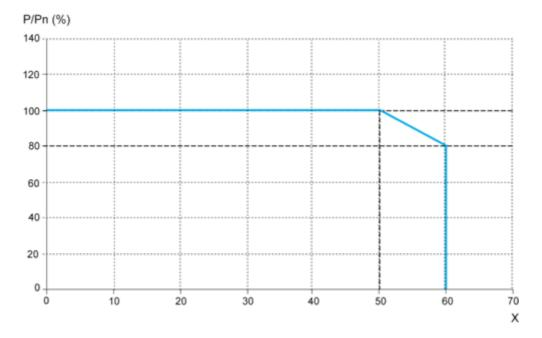
X Maximum operating temperature (°C) ABL 8RPM, ABL 8RPS, ABL 8WPS mounted vertically Derating should be considered in extreme operating conditions:
