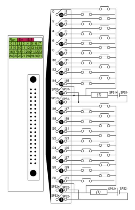
(1) fuse: fast blow fuse of 0.5 A for each 16-channel group power supply 24 VDC SPS sensor power supply
