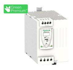
Regulated switch power supply, modicon power supply, 3 phases, 380...500V AC, 24V, 20A
