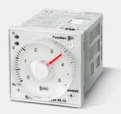
**Technical description:** Plug-in timers 8 A, Multi-function, 2 pole, 8 A, AC/DC coil, 230 V, operating from 20.4 to 264.5 V (AC)/(DC), rated power 2.5 VA (AC) / 1.5 W (DC), ambient temperature from -10 to +55 °C
