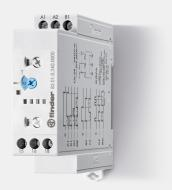
**Technical description:** Modular timers, Multi-function, 1 CO (SPDT), 16 A, AC/DC coil, 240 V, operating from 16.8 to 265 V (AC)/(DC), rated power 1.5 VA (AC) / 2 W (DC), Version: Standard, ambient temperature from -20 to +60 °C
