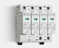
**Technical description:** Surge Protection Devices (SPD), Type 2, 4 varistors, Remote status signalling contact: Without remote status signalling contact, Nominal discharge current: 20 kA, AC supply version, nominal voltage 275 V,
