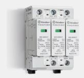
**Technical description:** Surge Protection Devices (SPD), Type 2, 3 varistors, Remote status signalling contact: Without remote status signalling contact, Nominal discharge current: 20 kA, DC supply version, nominal voltage 750 V.
