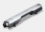
**Technical description:** LED light-1200 lumens, AC/DC supply version, nominal voltage 230 V, operating from 9.6 to 52.8 V (AC) and from 88 to 264 V (DC), rated power 9 VA, Switching via ON/OFF switch, Connections: Push-in terminals for the connection to a single unit, ambient temperature from -30 to +55 °C
