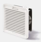
**Technical description:** Filter Fan – for indoor use, Enclosure cut-out: Size 1 (92 x 92) mm, Nominal air volume: 24 m3/h, Colour: Grey RAL 7035, AC supply version, nominal voltage 230 V, operating from 184 to 253 V, ambient temperature from -15 to +55 °C
