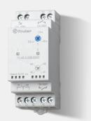
Technical description: Monitoring relays, Priority change, 2 NO, 12 A, AC/DC coil version, nominal voltage 230 V, operating from 90 to 264 V (AC)/(DC), rated power 3.9 VA (AC) / 1.5 W (DC), AqNi, Options: Max. 150 k $\Omega$ , ambient
