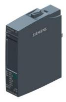
SIMATIC ET 200SP, TM count 1x 24 V Counter module, 1 channel for 24 V incremental encoder or pulse encoder, 3 DI, 2 DQ Suitable for BU type A0, packing quantity: 1 unit,
