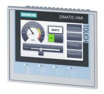
SIMATIC HMI KTP400 Comfort, Comfort Panel, key/touch operation, 4" widescreen TFT display, 16 million colors, PROFINET interface, MPI/PROFIBUS DP interface, 4 MB configuration memory, Windows CE 6.0, configurable from WinCC Comfort V11
