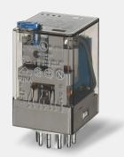
**Technical description:** Industrial relay, 8 and 11 pin plug-in socket version, 3 pole, CO (nPDT), 10 A, AqNi, DC coil, 24 V, operating from 19.2 to 26.4 V, rated power 1.3
