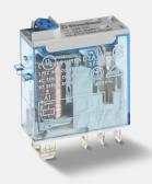
**Technical description:** Miniature Industrial relay, Spade/blade terminal Faston, 1 pole, C0 (nPDT), 16 A, AgNi, DC coil, 12 V, operating from 8.8 to 13.2 V, rated power 0.5 W, resistance 300  $\Omega$ , consumption 40 mA, holding voltage 4.8 V, must drop-out voltage 1.2 V, option: Lockable test button + mechanical indicator, ambient temperature from -40 to +70 °C
