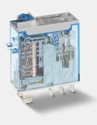
Technical description:Miniature Industrial relay, Spade/blade terminal Faston, 1 pole, CO<br/>(nPDT), 16 A, AgNi, AC coil, 230 V, operating from 184 to 253 V, rated<br/>power 1.2 VA, resistance 28000 Ω, consumption 5 mA, holding voltage<br/>184 V, must drop-out voltage 46 V, option: Lockable test button +<br/>mechanical indicator, ambient temperature from -40 to +70 °C
