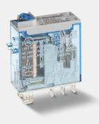
**Technical description:** Miniature Industrial relay, Spade/blade terminal Faston, 1 pole, CO (nPDT), 16 A, AgNi, AC coil, 12 V, operating from 9.6 to 13.2 V, rated power 1.2 VA, resistance 80 Ω, consumption 90 mA, holding voltage 9.6 V, must drop-out voltage 2.4 V, option: Lockable test button + mechanical indicator, ambient temperature from -40 to +70 °C
