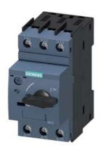
Special type Circuit breaker size S00 for motor protection, CLASS 10 A-release 4.5...6.3 A N-release 82 A screw terminal Standard switching capacity Ambient temperature -50  $^{\circ}\text{C}$  500 switching cycles
