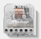
**Technical description:** Step relays, Screw terminals, Single pole switching -1 NO, 10 A, AC coil, 24 V, operating from 19.2 to 26.4 V, rated power 4.5 VA, resistance 70 Ω, consumption 180 mA, ambient temperature from -40 to +40 °C
