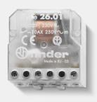
**Technical description:** Step relays, Screw terminals, Single pole switching – 1 NO, 10 A, AC coil, 12 V, operating from 9.6 to 13.2 V, rated power 4.5 VA, resistance 17  $\Omega$ , consumption 370 mA, ambient temperature from -40 to +40 °C
