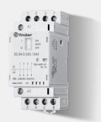
**Technical description:** Modular contactor, 25 A, 4 pole, NO, 25 A, AgSnO2, AC/DC coil, 24 V, operating from 19.2 to 26.4 V (AC)/(DC), rated power 2 VA (AC) / 2.2
