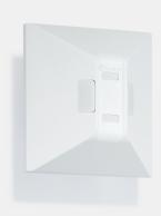
Technical description:Movement and presence detector, Movement detector wall mounting,<br/>Single pole switching, 10 A, Programming: Standard, Contact circuit:<br/>Volt-free output contact, AC supply version, nominal voltage 230 V,<br/>operating from 96 to 253 V, rated power 1.5 VA, ambient temperature<br/>from -10 to +50 °C
