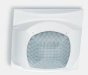
**Technical description:** Movement and presence detector, Movement and presence detector, Single pole switching, 10 A, Programming: Bluetooth, Contact circuit: Volt-free output contact, AC supply version, nominal voltage 230 V. operating from 96 to 253 V, rated power 1.5 VA, ambient temperature from -10 to +50 °C
