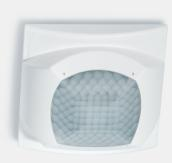
**Technical description:** Movement and presence detector, Movement and presence detector, Single pole switching, 10 A, Programming: Standard, Contact circuit: voltage output, Special version: Push-button connection, AC supply version, nominal voltage 230 V, operating from 96 to 253 V, rated power 1.5 VA, ambient temperature from -10 to +50 °C
