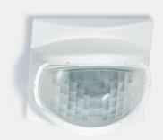
**Technical description:** Movement and presence detector, For corridors, Single pole switching, 10 A, Programming: Standard, Contact circuit: Volt-free output contact, AC supply version, nominal voltage 230 V, operating from 96 to 253 V, rated power 1.5 VA, ambient temperature from -10 to +50 °C
