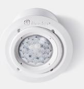
**Technical description:** Movement and presence detector, Indoor ceiling installations – recessed mounting, Single pole switching, 10 A, Programming: Standard, Contact circuit: voltage output, AC supply version, nominal voltage 230 V, operating from 96 to 253 V, rated power 2 VA, ambient temperature from -10 to +50 °C
