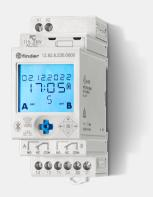
**Technical description:** Time switch, Annual "Astro", Bluetooth 5, NFC programming, 35 mm wide, 2 CO (DPDT), 16 A, AC/DC supply version, nominal voltage 230 V, operating from 88 to 253 V (AC)/(DC), rated power 2.8 VA (AC) / 0.9 W (DC), ambient temperature from -20 to +50 °C
